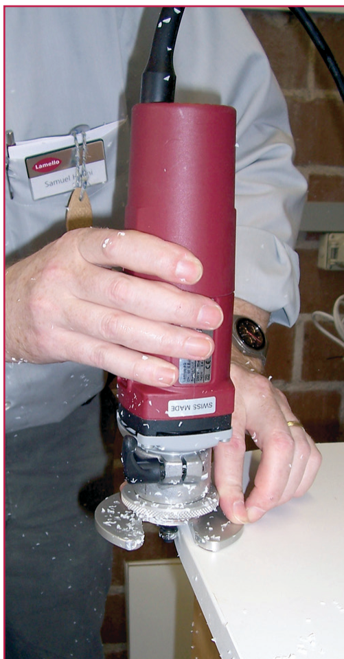
Variable tool opening, 25mm or 34mm depending on the cutter size.
