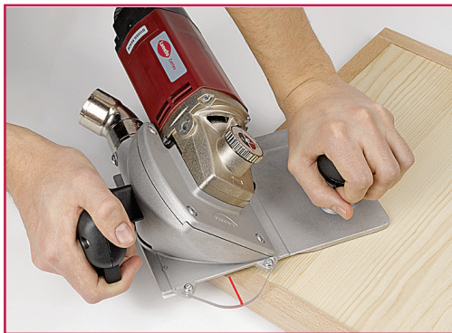
Flush-planing efficient and clean
