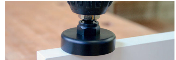
Installation with insertion jig
